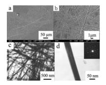
Ultralong orthorhombic  $V_2O_5$  nanowires were synthesized by a facile hydrothermal oxidation route. Further research proves that there are certain criteria for the selection of suitable oxidizers. The optimal oxidizer should not only be thermodynamically favorable, but also kinetically favorable.
